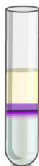
The formation of a purple ring is a positive indicator for Molisch's Test
